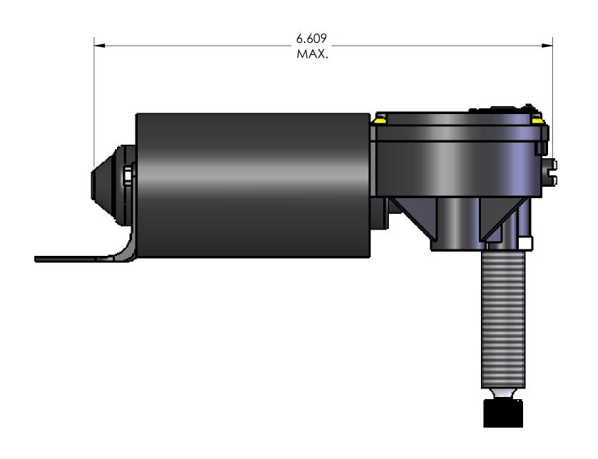
**SPECIFICATIONS:** VOLTAGE-12:24 WEIGHT-APPROX. 3 LBS. CURRENT STALL-16 1/2 AMP- NO LOAD-1 AMP STAFF TORQUE-95 IN. LBS. SPEED-60 RPM-NO LOAD FOR 12 VOLT MOTORS USE 4 AMP FUSE FOR 24 VOLT USE 3.5 AMP FUSE
